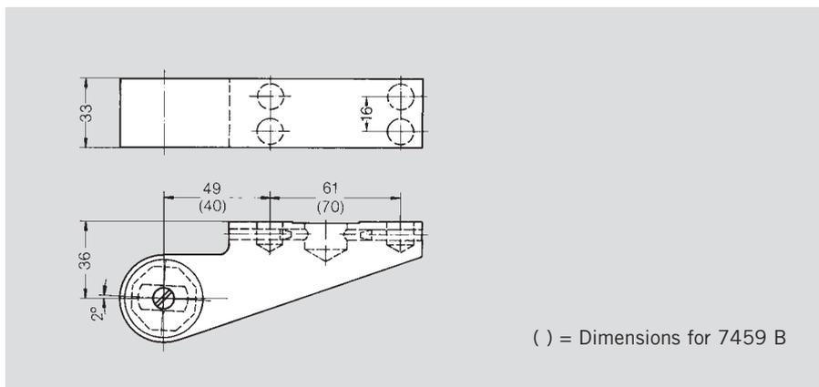
**Drill jig for aluminium hinges**
